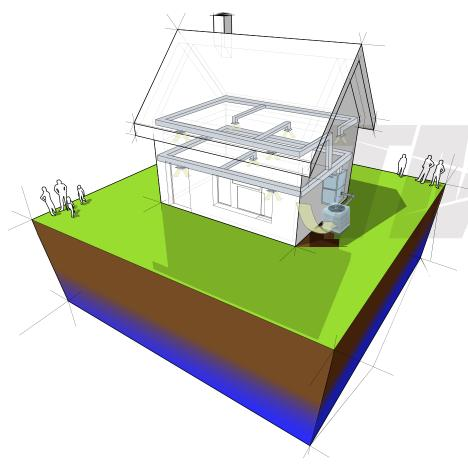
**Air-source heat pumps** are the most common type. They absorb heat from outdoor air using an outdoor unit. Refrigerant circulates through the system, and as it passes over the outdoor coil, it absorbs heat from the air. Air-source heat pumps are relatively easy and cost-effective to install since they don't require extensive excavation.
