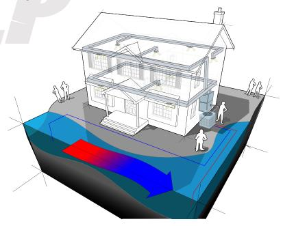
**Water-source heat pumps** work similarly but extract heat from a water source, such as a lake or pond. This kind of heat pump is efficient and is a viable option in areas with access to a nearby body of water.
